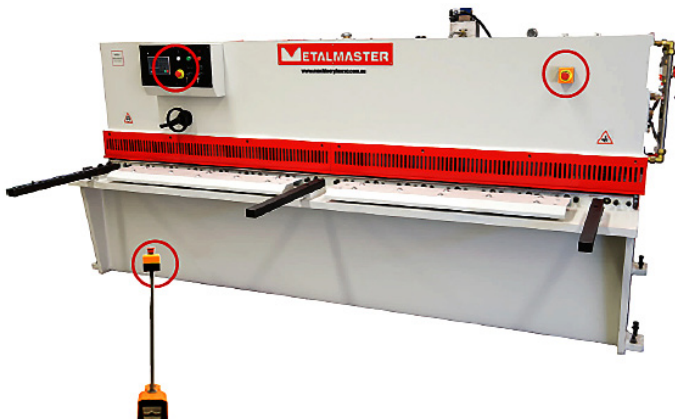
Emergency Stop Buttons
